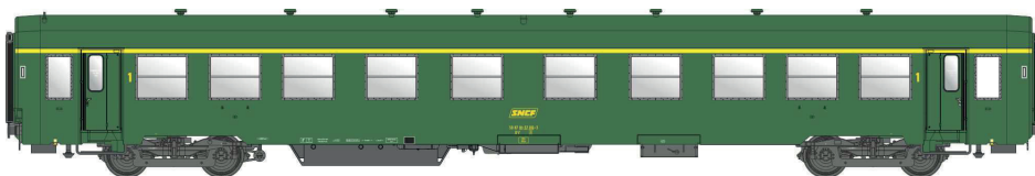
MW40042 A4t4 U63 bogies Y24
